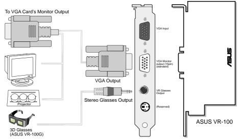
When using a Y-type cable, you do not need to connect the VGA Input of the VR-100 to your VGA card's monitor output (see diagram above).
